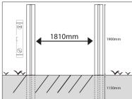
Insert the posts in the middle of the hole, using a spirit level. Make sure they are completely vertical and straight.
