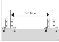
The posts should be spaced at 1810mm internal to internal distance
