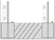
Use a spirit level and make sure the posts are completely vertical and straight again.
