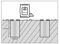
Pour the concrete into the hole until it's 600mm below the ground level.Fill the top of the hole with soil once the concrete is set.
