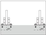
Make sure the steel base is 90 degree vertical to the ground.
