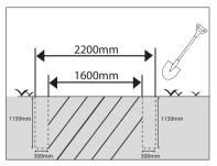
Use a shovel to dig a hole with 300×600mm minimum size. The hole should be spaced at 2200mm out-to-out distance and 1600mm internal to internal distance.
